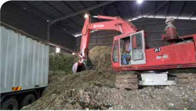
**Loading of Alternative Fuel for transport to the kiln.**
